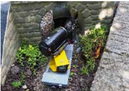
iPhone mounted on the camera wagon using the adaptor from a selfie stick.
