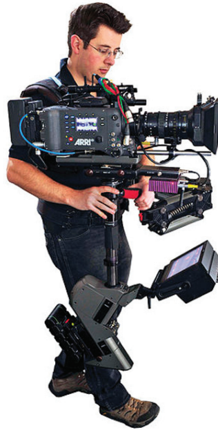
Above: Steadicam Operator John Fry with Master Steadicam flying Arri Alexa HD digital cinema camera and Angenieux PL mount zoom lens*
